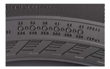
The location and pressure indicators on the sidewall info area improve safety. The information area allows for recording the correct inflation pressure and installation location during tyre change. Safety and comfort are improved further by a new section that can be used to record the tightening torque of the wheel nuts for alloy wheels. The correct tyre pressure makes driving safer and steering more responsive, reduces tyre wear and saves fuel.
