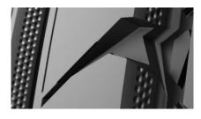
Several new innovations provide added safety for sudden rainfalls, which are an essential part of the Central European summer. The bullet-shaped Trumpet Grooves store water from between the tyre and the road, accelerating its flow from the main grooves towards the transverse grooves and maximising grip even on rain-soaked roads.
