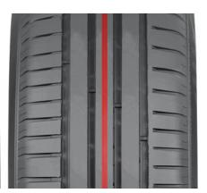
The next-generation Driving Safety Indicator on the centre rib indicates tread depth. You can check the amount of remaining tread in millimetres by examining the row of numbers on the tread. The numbers and water drop symbol indicating a risk of aquaplaning disappear, as the tyre wears down. When the tread depth is below 4 mm, a red stripe that indicates low tread depth will appear around the tyre. When this happens, please purchase new summer tyres in order to ensure maximum safety.
