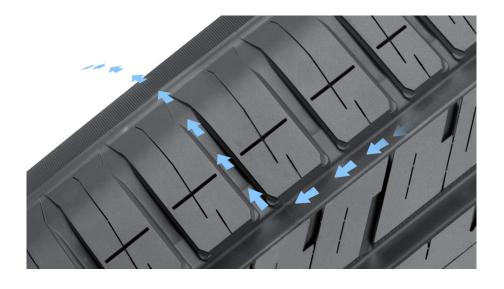
The Nokian Tyres Coanda Technology accelerates the removal of water from the longitudinal groove and effectively prevents aquaplaning. The curved, ramp-like design of the tread blocks on the inner shoulder guides and accelerates the flow of water from the longitudinal groove into the transverse groove. The Coanda effect denotes the tendency of flow to turn towards a nearby surface. The
