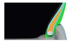
The special clinch rubber compound on the bead area flexibly presses against the wheel flange, avoiding possible abrasion under heavy use. This compound innovation improves durability but also helps tyre fitment. The innovation also effectively minimises the interior noise, since it dampens the vibrations from the tyre body, preventing them from passing into the tyre and further inside the vehicle.
