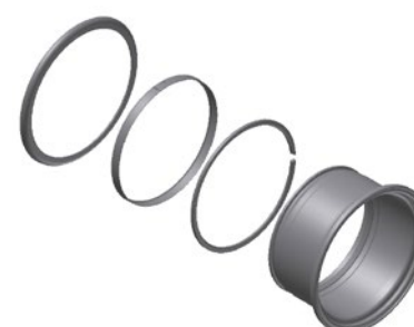
› 4-piece rim / bead seat ring and lock ring the same component
