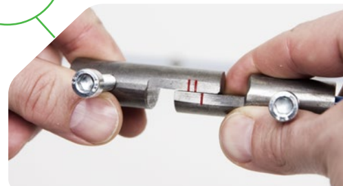
Mandrel gauge for rim circumference measurement
