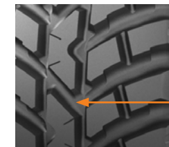
Nokian TRI 2 tread depth measuring point on top of tie-bar
