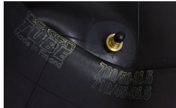
Size designation marking on tube
