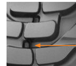
Nokian Forest King F2 tread depth measuring point beside tie-bar
