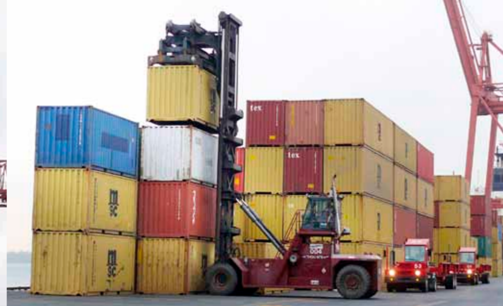
Nokian HTS tyres stabilise reach stackers that handle stacks of up to four containers.
